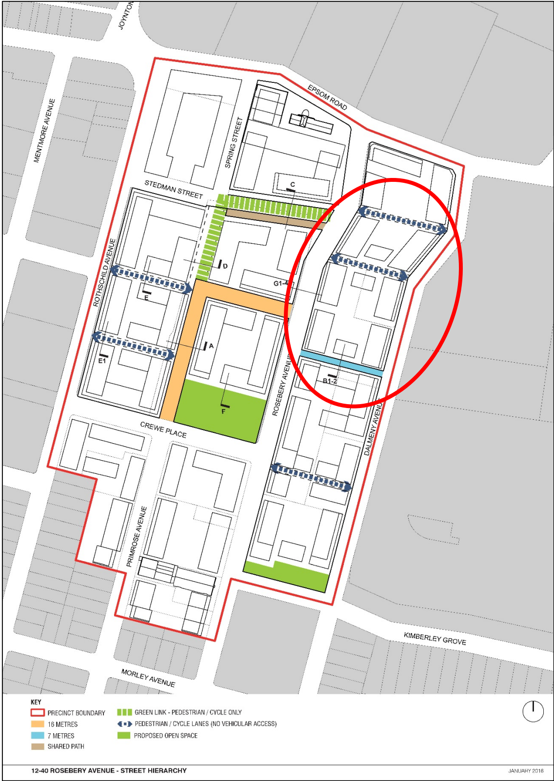
Figure 5.171: North Rosebery Street Hierarchy and Street Sections
